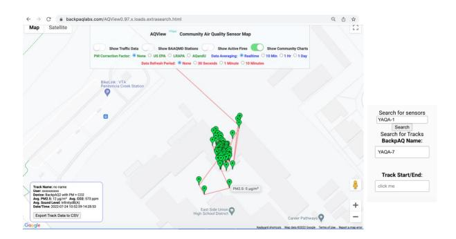
You can click on any marker to see the PM2.5 values at that point. Additionally, the red lines which connect the markers indicate the path taken.
